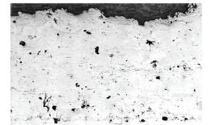
Optical micrograph at 100x of a typical SHS7570W coating
