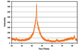
The broad amorphous hump is indication that the as-sprayed SHS7570W coating structure is a metallic glass
